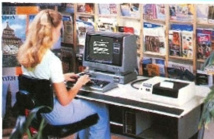
Mini-disk for expanded language, fast data handling and approximately 49,900 bytes of user disk storage space. Quick Printer provides 80 column hard copy and program listings. System Desk holds the entire system with plenty of work space left over.
